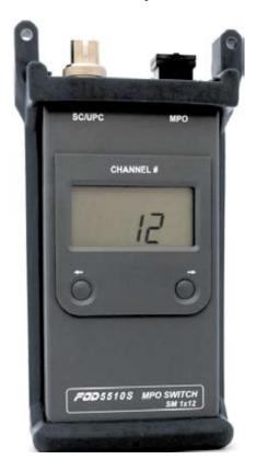
The FOD 5510 Series Fiber Optic Switches are a compact, robust, battery operated **1X12** or **1X16** switch designed specifically for use with OTDRs and Optical Loss Testers for certifying, testing and troubleshooting MPO terminated cables and harnesses. Whether used in manual mode with pushbutton controls, or automated with USB Windows® or Linux® based remote control drivers, the FOD5510 Series brings multi-fiber testing to a new level.
